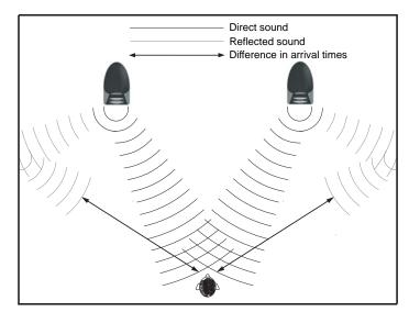
Figure 2. Optimum placement for reducing reflection problems
